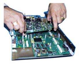
If another 6KPM card is replacing the one that has been removed, follow the steps as described for installing a 6KPM card discussed in Section 3.7.1.
